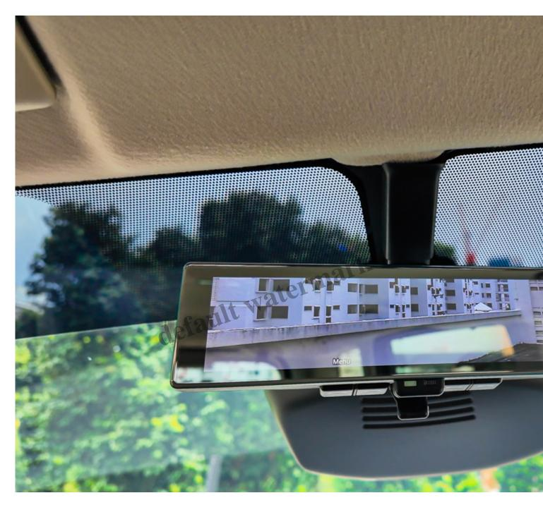
The Intelligent Rear View Mirror offers the option of a digital view, ensuring a clear and unobstructed view of what's behind, even with a full load of passengers or cargo.
