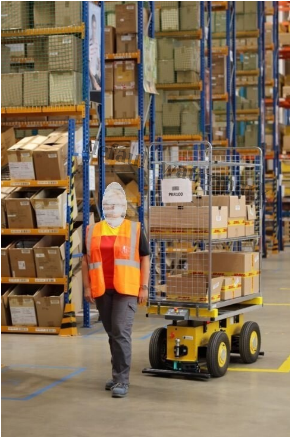
TAG Industrial's EffiBOT can follow a worker, lead ahead or run autonomously. Image: TAG Industrial
