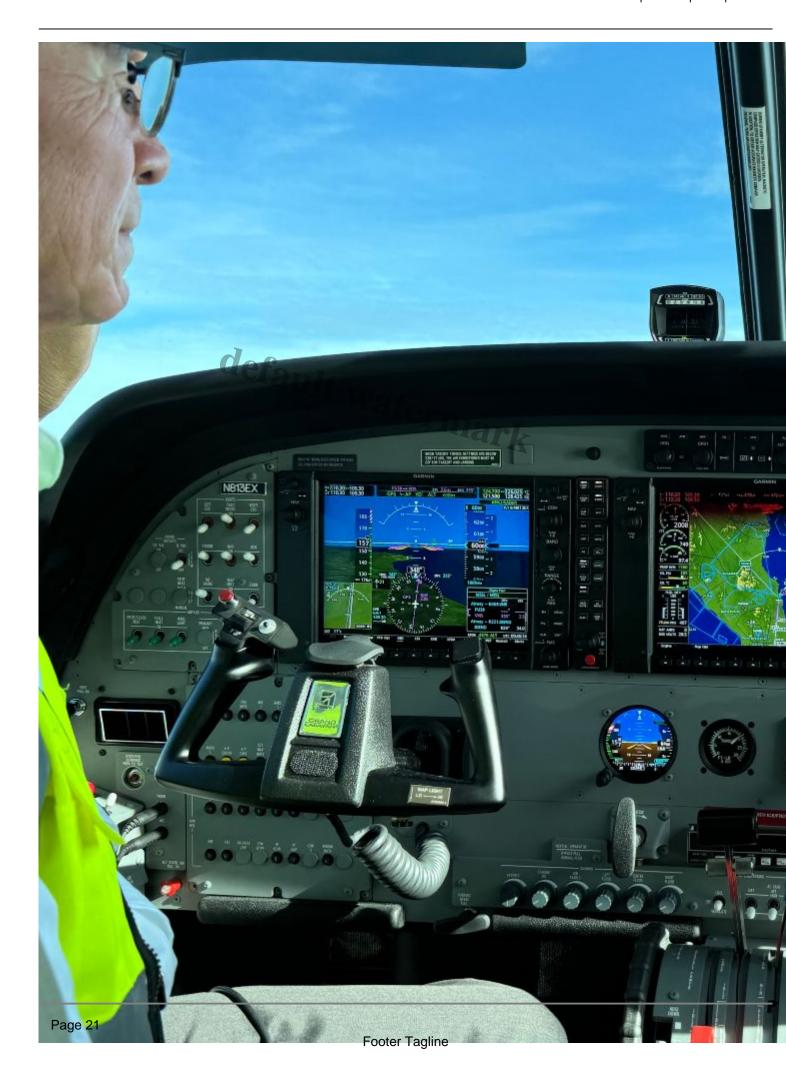
Its state-of-the-art control panel is truly one of its kind. A fully integrated flight deck features the Garmin G1000 NXi at its core. Its high-resolution displays and intuitive graphical interface enhance situational awareness and boost operational efficiency. The optional Garmin® enhanced automatic flight control system (E-AFCS) includes Electronic Stability and Protection (ESP), Underspeed Protection (USP), and an emergency descent mode.
